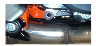
The size of tap needed to add threads to the engine case is a 10mm x 1.5. The recommended drill for this thread tap is 8.5mm and must be used before the tap is inserted to prevent case damage. Only drill into the case 35mm from the outside edge of the frame mount. \*Reminder - this should only be done if mounting a PowerParts Skid Plate assembly
