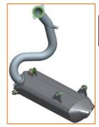
**Innovative Underfloor-exhaust system** positioned close to the centre of gravity leads to a weight distribution of 51.5% (front) and 48.5% (rear) which helps to reach the superb rideability
