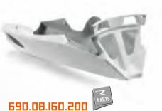
FIBERGLASS UNDER-ENGINE FAIRING
