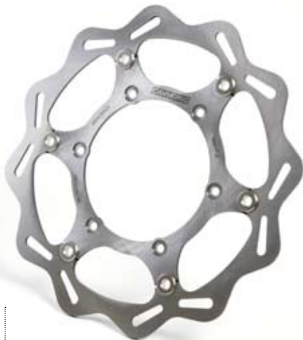
Front brake disk Nambotin Replica 2010 Ref.: BE52000R3010
