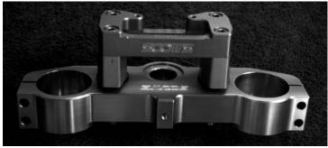
6061 Aircraft Aluminum triple clamps complete with matching barclamp to mount our damper. Increased clamping area, reduced flex, optional bar mounting positions and anodized for long term usage. Available for most late model bikes. This insures proper mounting alignment, a common problem with other brand triple clamps.
