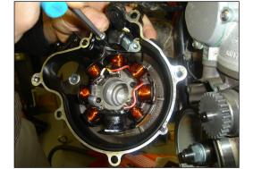
Use the new ignition cover gasket provided in the kit when mounting the ignition cover.
