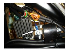
Connect the two wires along with the ground wire from the wiring harness to the mount that holds the igntion coil to the frame.
