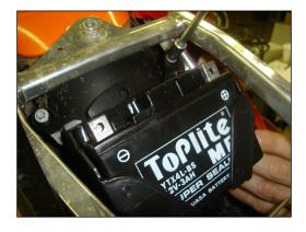
Use the three EJOT PT screws (p.n.0017060203) to mount the battery box in the airbox.
