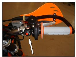
Mount the e-starter button on the right side of the handlebar.
