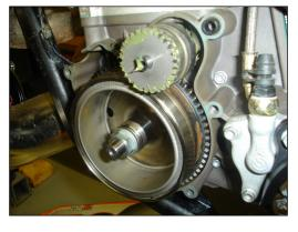
Mount the stator and pulser coil in the new ignition cover. Use loctite 243 on the stator and pulser coil bolts.
