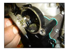
Prepare the intermediate shaft (p.n.55140022000) for mounting by lightly coating the gear and the shaft with grease.
