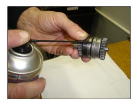
Prepare the bendix for mounting by spraying some light penetrant oil on the bendix spring.
