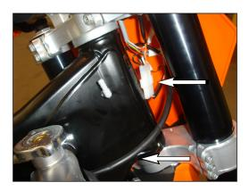
Route the plug of the wiring harness that plugs into the e-starter button towards the front of the motorcycle and through the space between the frame and radiator.
