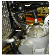
Connect the starter cable to the starter using the self locking nut (p.n.0985060003) supplied in the kit.
