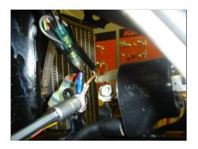
In preparation to mount the voltage regulator and wiring harness, remove the screw that connects the two wires to the frame. The voltage regulator will attach to this frame mount.
