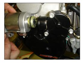
Lightly grease the starter shaft and o-ring and insert it into the ignition cover for mounting.
