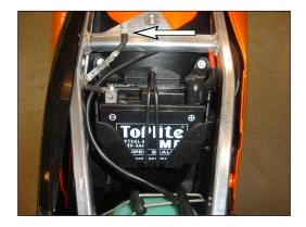
Connect the ground cable to the pre-drilled hole in the subframe using the contact washer (p.n.58411098100) and the 6x10 HH collar screw (p.n.0025060106)
