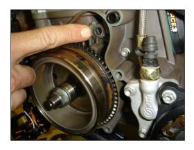
Then mount the bendix assembly into the existing hole in the engine case.
