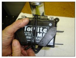
Prepare installation of the battery box, battery and rubber hold down strap.
