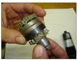
Apply grease to the bendix gears.
